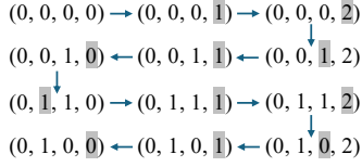
Fig. 6: Reuse-aware traversal over shard bucket-ID assignments. Adjacent iterations differ in exactly one dimension.
